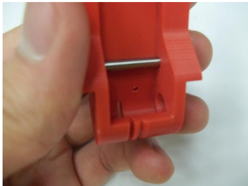
1. Drill hole for torsion spring stem. A divot for this should be incorporated into the CAD
