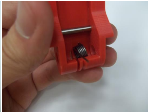
2. Insert one stem of the torsion spring into the drilled hole
