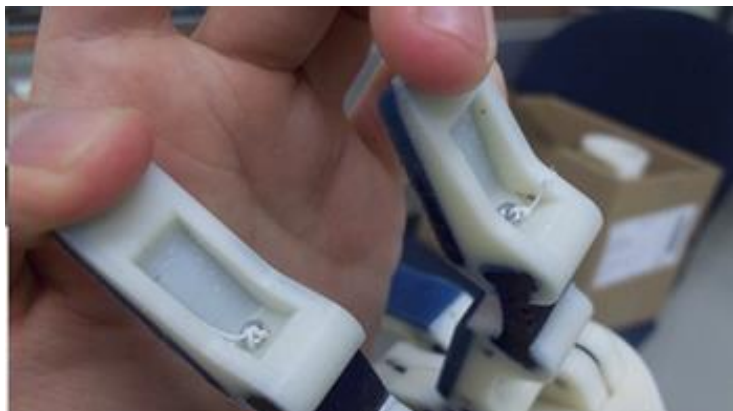
- Using a nut to terminate the tendon
