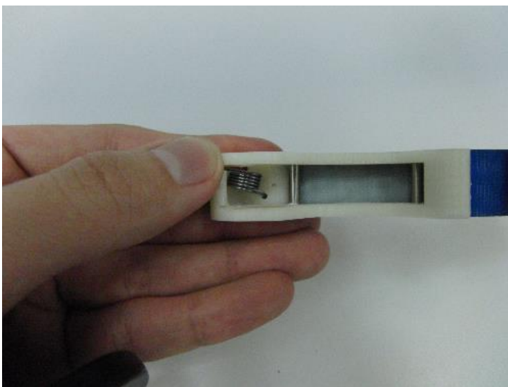
1. Insert torsion spring stems into slot and offset hole clearance
